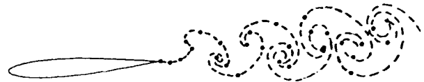
Fig. 8 Positions of vortex cores in the wake behind a sinusoidally ( \omega = 17 ) heaving airfoil.
